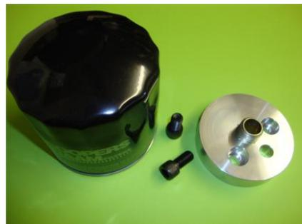
Clean the area around the filter head and then remove the two bolts or studs which hold the filter head onto the block. Remove the filter head completely, including the bowl and filter. Clean the engine block where the filter head was located and remove the old gasket. Ensure that the mating surface is clean and dry.
